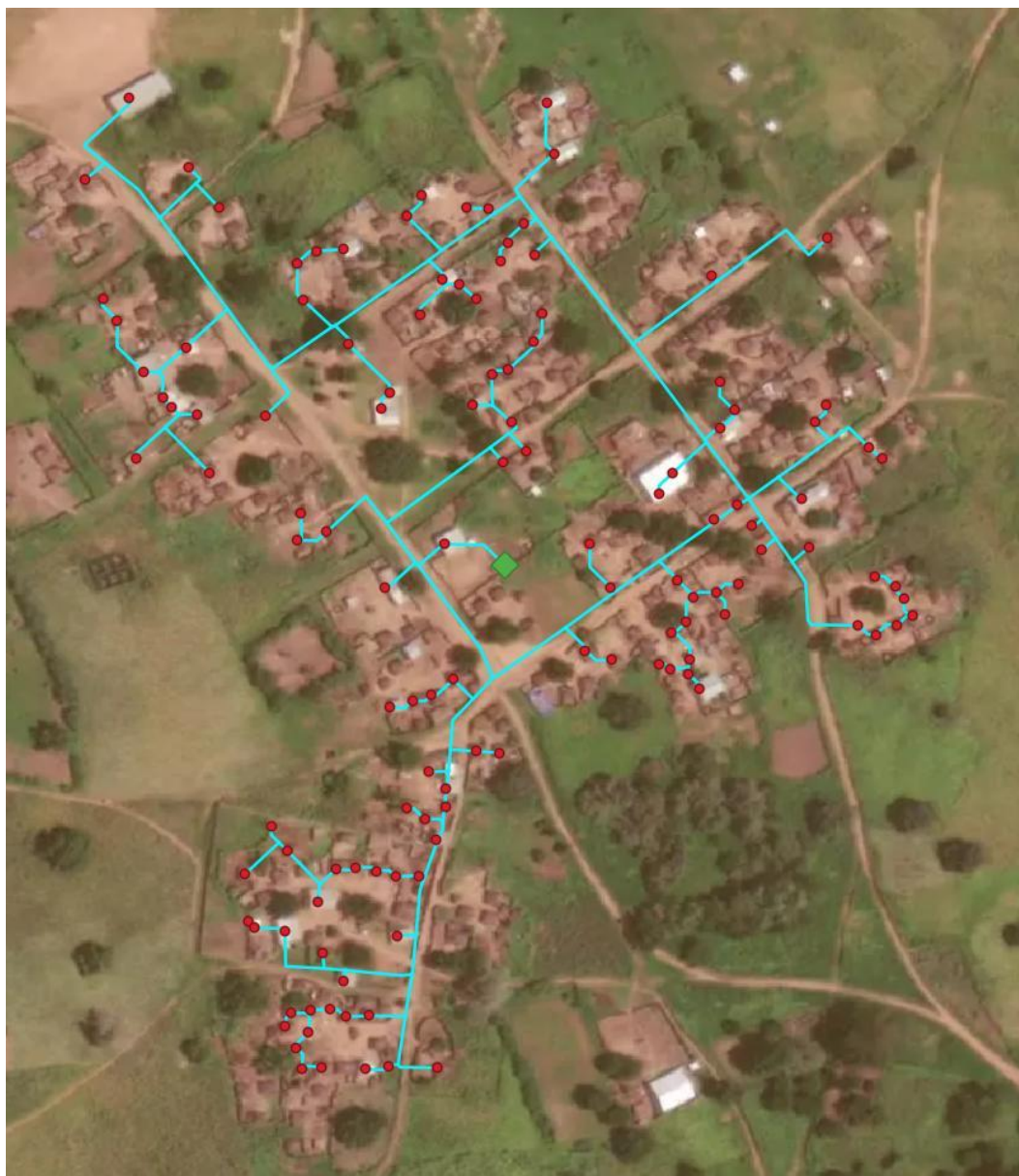
Figure 23: Results of the Pathfinder algorithm, used to estimate a cable length required to deploy a replicated microgrid.
